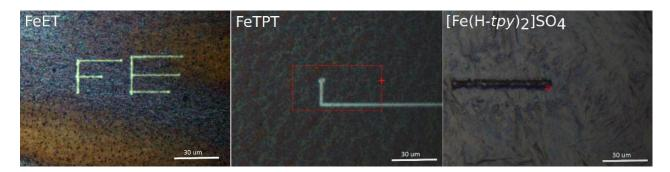
**Figure 9.** Optical microscopy images of films of two phosphole Fe-MSPs and  $[Fe(tpy)_2]SO_4$  showing traces drawn by a 532 nm laser beam with a power of 5 mW.
