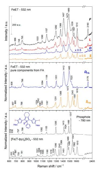
**Figure 5.** Comparison of relevant RS: (**Top**): the first (F) and last (L) RS of the **FeET** (532 nm) series and RSs of the disappearing (D) and stable (S) components obtained by the subtraction method; (**Middle**): pure spectral components obtained by factor analysis (FA) of the whole spectral set; (**Bottom**):off-resonance RS of the precursor central unit and RRS of [Fe(T-tpy)<sub>2</sub>]SO<sub>4</sub> complex (T-tpy stands for 4'-(2-thienyl)terpyridine).
