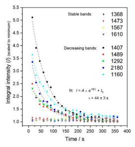
Figure 7. Time evolution of individual Raman bands of FeET exposed to the excitation radiation.
