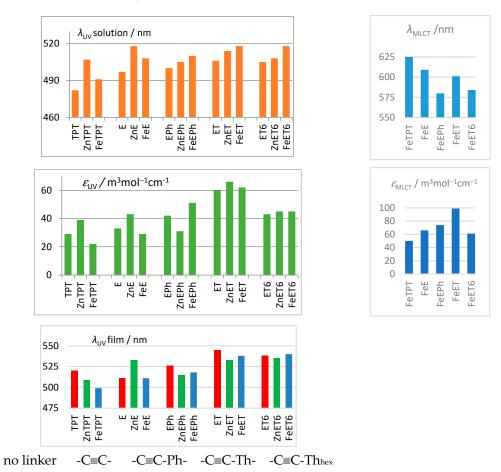
Figure 2. Effect of the linker structure on the UV/vis characteristics of unimers and MSPs.
