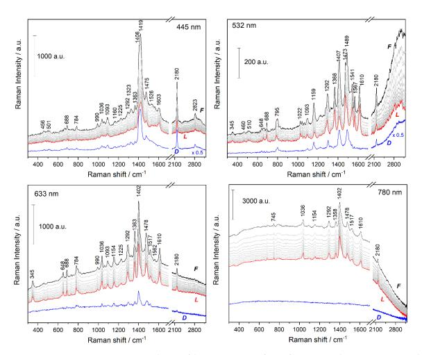
**Figure 4.** Time evolutions of the Raman spectra of **FeET** films measured using various  $\lambda_{\rm exc}$ . Black—first RS (F); red—last measured RS (L); blue (D = F - L)—difference spectrum. Accumulation time 15 s; total time 6–9 min; laser power at the sample: 0.1 mW for 532 and 633 nm and 5 mW for 445 and 780 nm.
