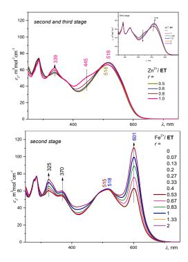
**Figure 1.** The UV/vis spectral changes accompanying assembly of  $Zn^{2+}$  (**up**) and  $Fe^{2+}$  (**down**) ions with unimer **ET** at mole ratios r from 0 to ca 0.5 (**left**) and at r > 0.5 (**right**).
