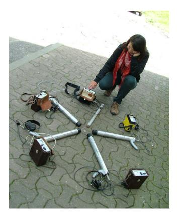
**Figure 1.** Comparative measurement of RP scintillometers at the field base in Lázně Libverda, Claim #3. Photo by Zdeňka Petrová September 2010, with permission.
