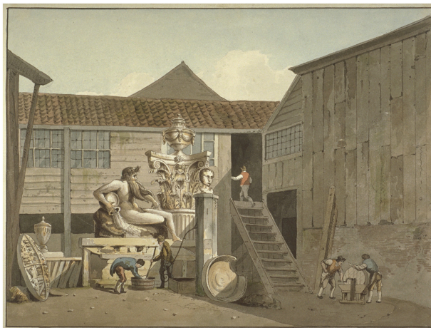
FIGURE 1 The work yard of Coade's artificial stone manufactory, Lambeth, c.1800. Note the workmen grinding and mixing raw materials (London Metropolitan Archives © City of London)
